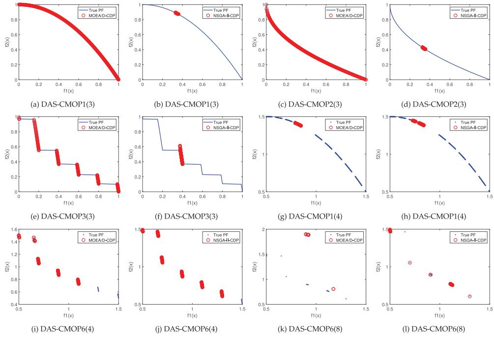
Figure 7: The feasible and nondominated solutions with the median  $IGD$  values in 30 independent runs by using MOEA/D-CDP and NSGA-II-CDP on DAS-CMOP1-3 and DAS-CMOP6 with different difficulty triplets. (a)–(f) show the populations achieved by MOEA/D-CDP and NSGA-II-CDP on DAS-CMOPs with convergence-hardness. (g)–(l) show the populations achieved by MOEA/D-CDP and NSGA-II-CDP on DAS-CMOPs with simultaneous diversity-, feasibility-, and convergence-hardness.
