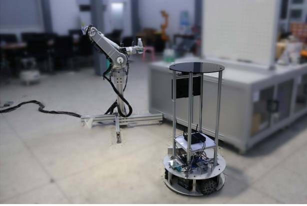
Fig. 7. Experimental environment: StellaX observes the position of the object and shares the information with the manipulator through the Intel NUC. After the manipulator performs the grasping task and places the object on the top of StellaX, autonomous navigation application will be execution.
