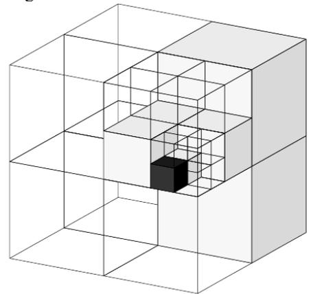
Fig.6. An example of an octree voxel structure and occupied (black) cells.
