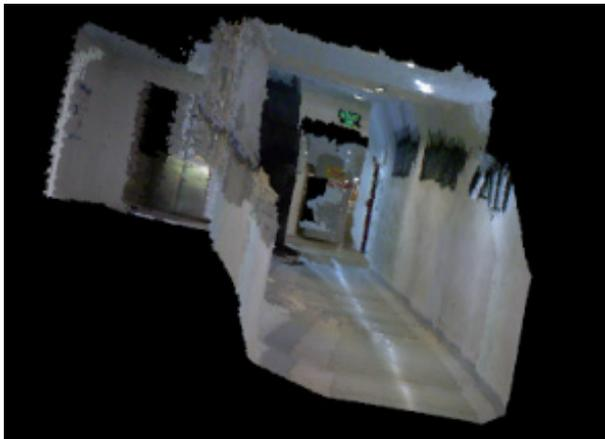
Fig.9. The 3D map synchronized mapping with 2D map by three wheels Omni-directional mobile robot.
