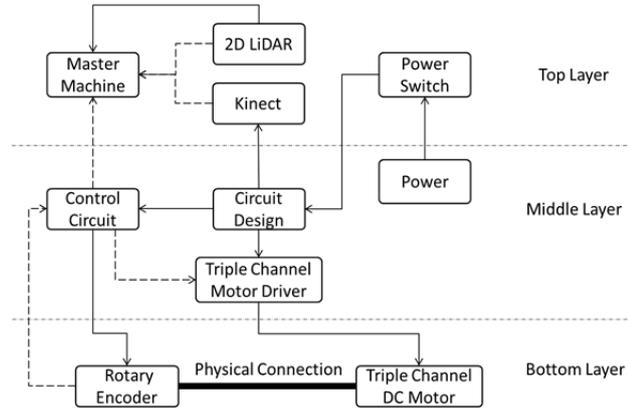
Fig.3. The connection of the subsystems.
