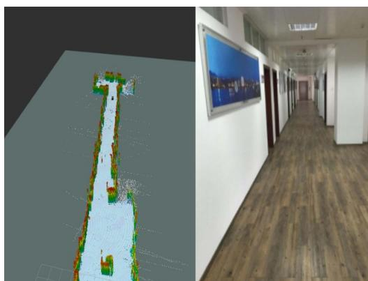
Fig. 14. Simultaneous construction of 2D grid map and OctoMap
