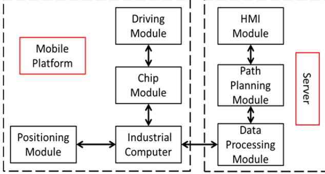
Fig.2. Block diagram of the mobile robot platform.
