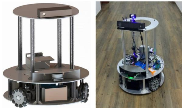
Fig.1. The prototype of the three wheels Omni-directional mobile robot.
