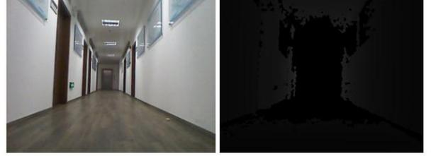
Fig.4. Color images and depth images obtained by kinect.
