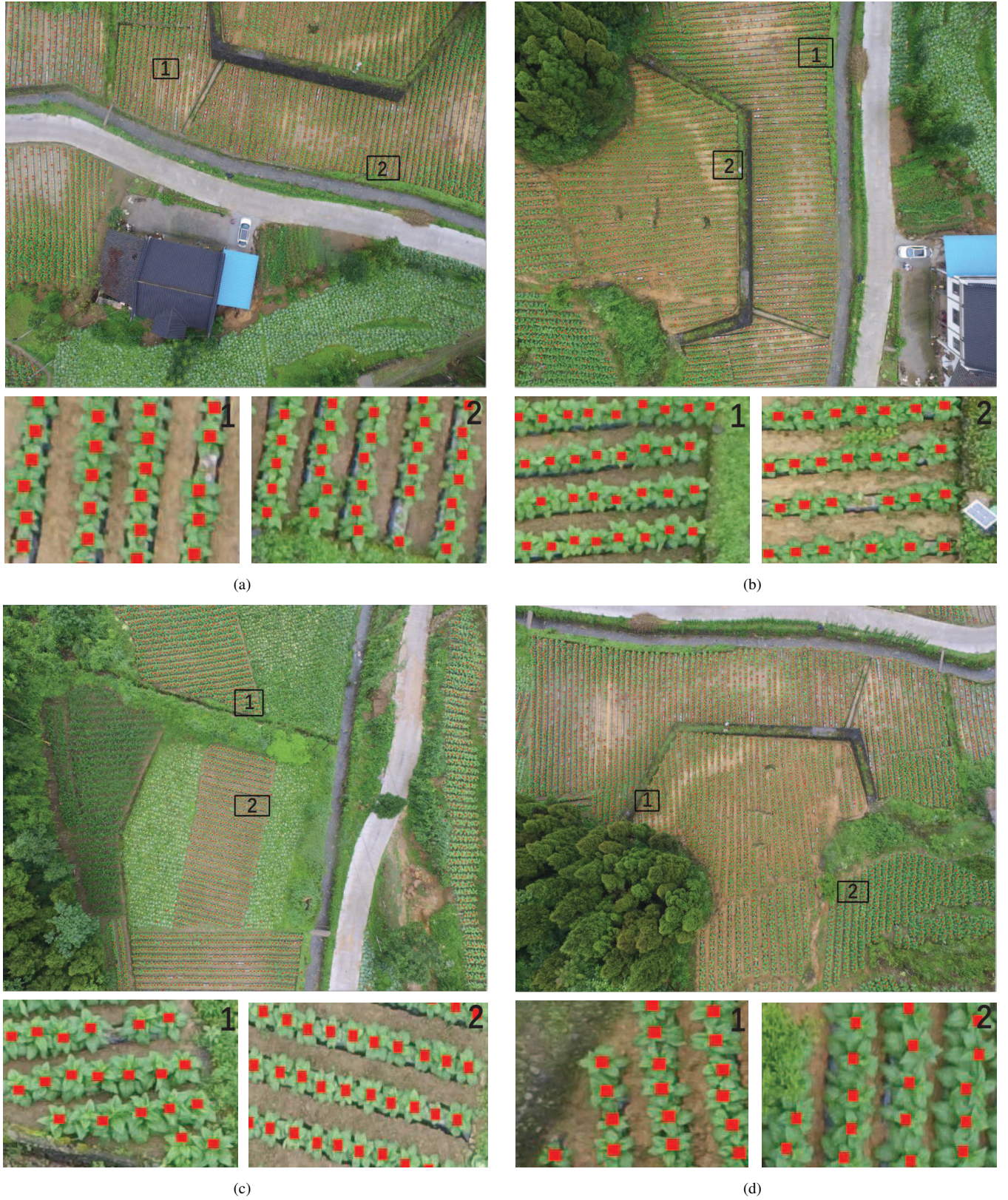
Fig. 11. Final tobacco-plant-detected images (Red regions represent the central regions of the detected tobacco plants. Black rectangles include the enlarged fragments of the images): (a) The first test image. The geo-coordinate of this image is ( N29^{\circ}29' 9.2094'' , E107^{\circ}40' 51.3395'' ). (b) The second test image. The geo-coordinate of this image is ( N29^{\circ}29' 10.0000'' , E107^{\circ}40' 51.1483'' ). (c) The third test image. The geo-coordinate of this image is ( N29^{\circ}29' 11.0611'' , E107^{\circ}40' 53.0032'' ). (d) The fourth test image. The geo-coordinate of this image is ( N29^{\circ}29' 10.5399'' , E107^{\circ}40' 50.8106'' ).
