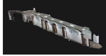
Figure 5. 3D indoor corridor map based on Monte Carlo localization in 2D map
