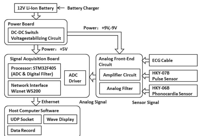
Fig.1. The architecture of the multichannel biomedical signal acquisition system
