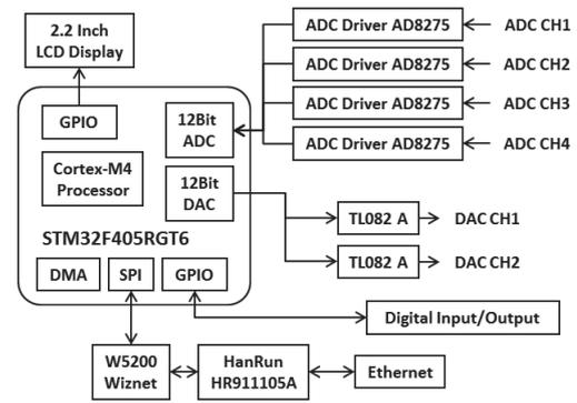
Fig3. The block diagram of Signal Acquisition Board
