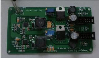
Fig.10. The power board
