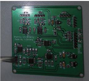
Fig.12.The signal front-end processing board
