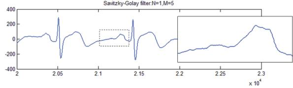
Fig.9. The Result of Applying Savitzky-Golay Filter to a Real ECG signal
