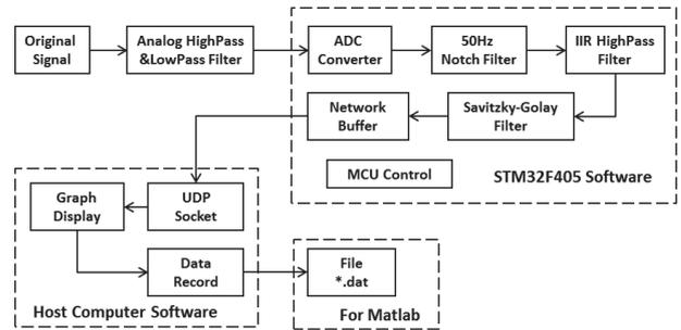
Fig.4.The signal flow diagram
