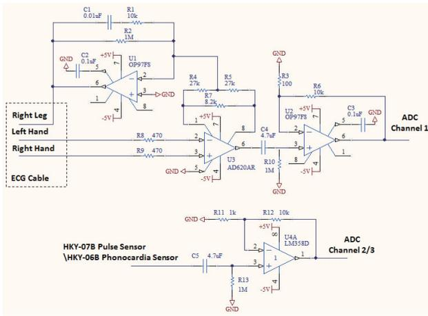
Fig.2.The Schematic Diagram of the Analog Front-End Circuit
