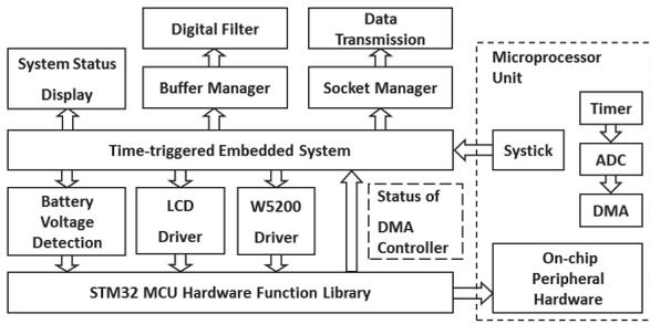
Fig.5.The Block Diagram of the Embedded System on STM32F405RGT6 Processor
