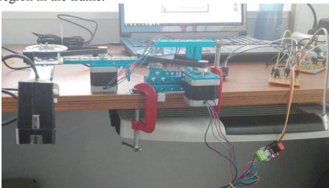
Figure. 6. The experimental setup with the robotic arm on which the video camera was mounted on. The arm could pan along the horizontal axis while vibration motors along the arm would simulate real-life distortions.
